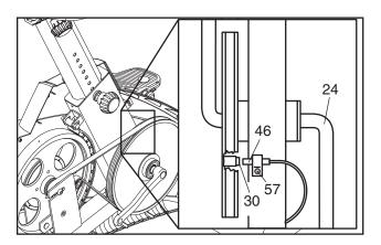
Turn the right crank arm for a moment. Repeat until the console displays correct feedback. When the reed switch is correctly adjusted, reattach the right side shield, the seat post knob, and the right pedal.
